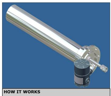
The Canty Direct Insertion Camera is designed for optimal image quality that is achieved by placing a camera as close to the process as possible. camera is placed within the insertion tube reducing lens length and reducing loss of image quality. The increase quality is ideal for applications that need very high picture quality and that need insertions up to 36" (914mm) in length.
