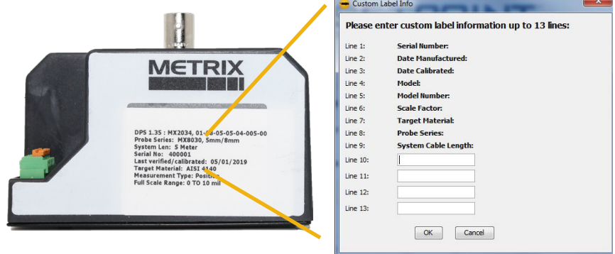
A user-generated label can be printed in the field with all device characteristics as well as user-specific tagging and installation particulars.
