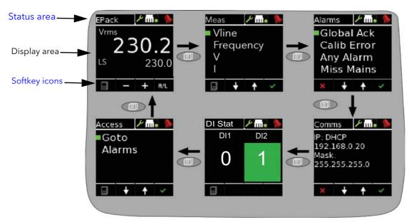
Figure 12 Operator interface
